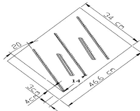
Figure 12: Fin distribution on condenser surface
