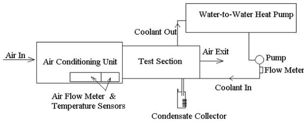
Figure 4: Experimental set up schematic diagram
