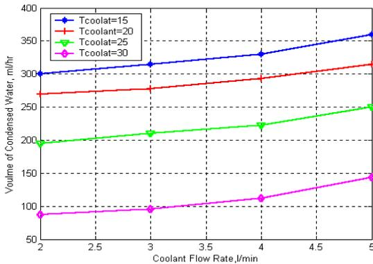
Figure 10: Effect of coolant temperature on condensate yield at air inlet conditions of  $T_{db}=44$  °C, 100% relative humidity at constant air velocity 0.2 m/s.
