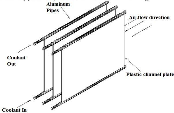
Figure 7: Plate channel condenser arrangement.
