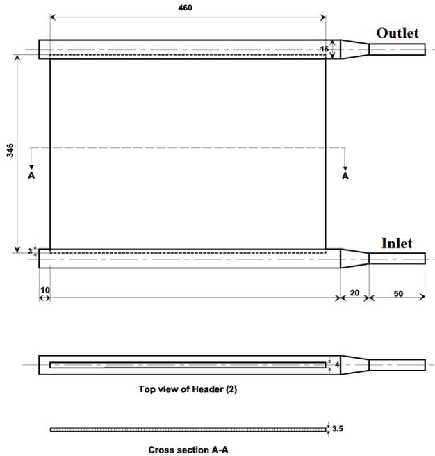
Figure 5: Plate channel condenser module
