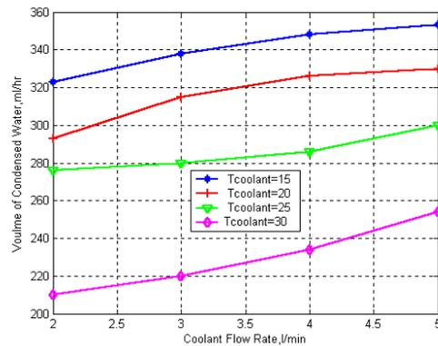
Figure 9: Effect of coolant temperature on condensate yield at air inlet conditions of  $T_{db}=55$  °C, 53% relative humidity at constant air velocity 0.2 m/s.
