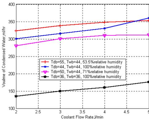
Figure 8: Water condensate production at constant coolant temperature of 15 °C and constant air velocity of 0.2 m/s
