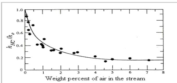
Figure 3: Effect of air on condensation heat transfer [5].
