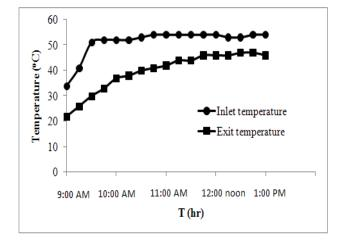
Fig. 8: The inlet and the exit thermal fluid (water) temperatures in the evaporator.
