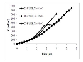
Fig. 3: Cumulative volume of desalinated water at different time of the year using water as a thermal fluid.
