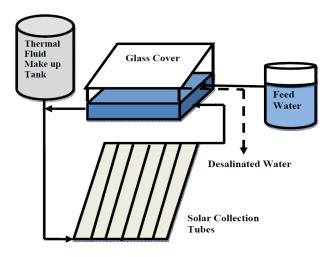
Fig. 1: A schematic diagram of the experimental setup.
