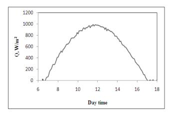
Fig. 2: Typical solar irradiation intensity versus day time in Irbid-Jordan.
