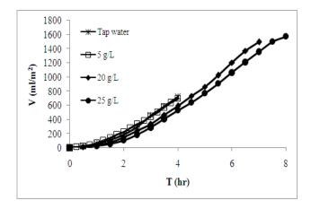
Fig. 7: The effect of feed water salinity on the productivity of the unit.
