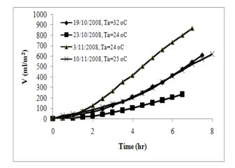
Fig. 4: Cumulative volume of desalinated water at different time of the year using jojoba oil as a thermal fluid.
