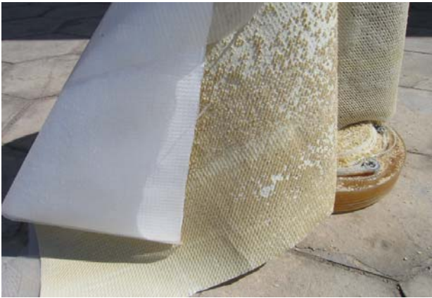
Fig.10. View of the membrane surface after 6 months of operation
