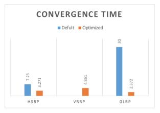
Fig. 22. FHRP Convergence Time Comparison
