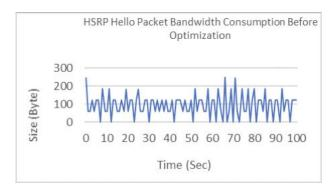
Fig. 5. HSRP Hello Packet Consumption without Optimization
