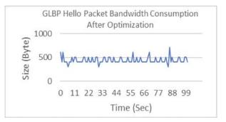
Fig. 18. GLBP Hello Packet Consumption After Optimization
