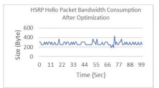
Fig. 6. HSRP Hello Packet Consumption with Optimization
