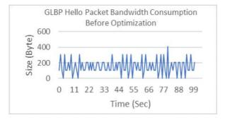
Fig. 17. GLBP Hello Packet Consumption Before Optimization
