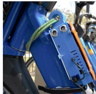
Fig. 1 - Multi-sensor mobile device mounted on a bicycle
