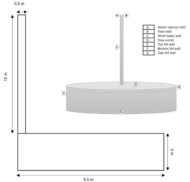
Fig. 1: Geometry of the axisymmetric greenhouse with wind tower integration (0° slope).
