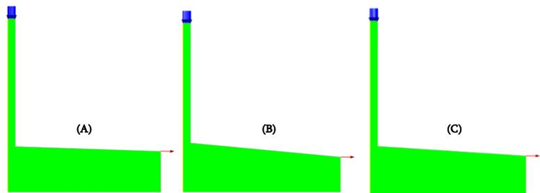
Fig. 3: Baseline mesh for the greenhouse a. 0.33/9° slope, b. 0.5/9° slope and c. 0.66/9° slope.
