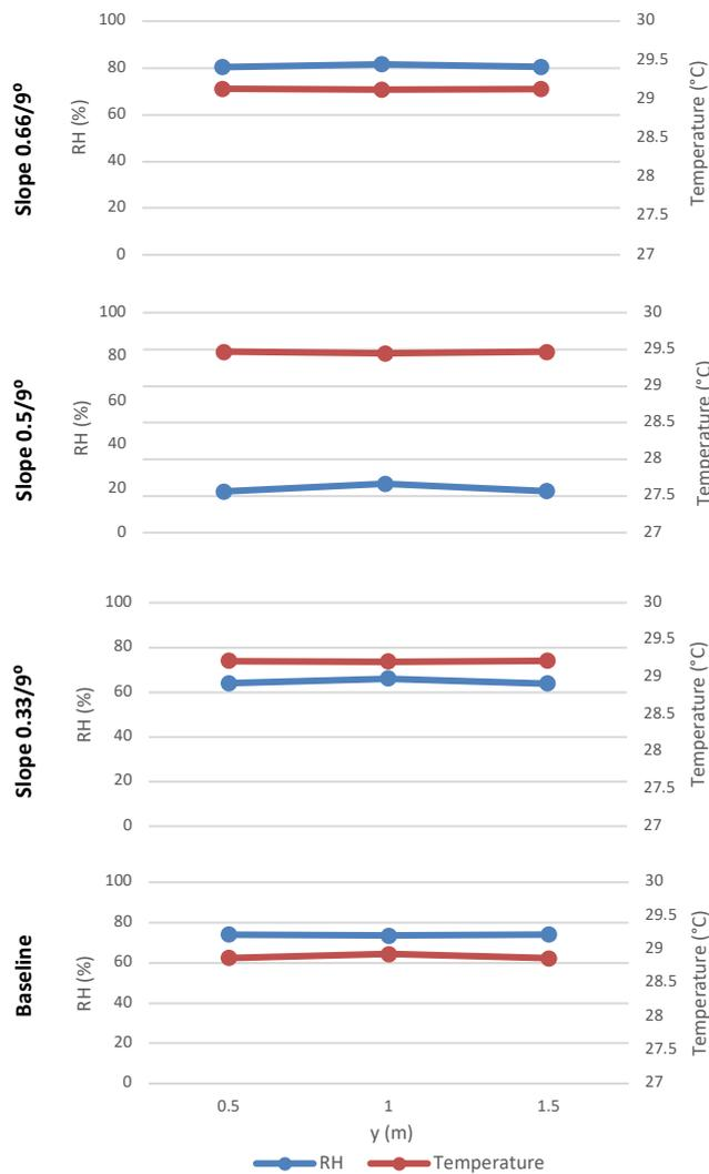
Fig. 10: Plot for the obtained temperature and relative humidity values at selected heights of the four greenhouses studied.
