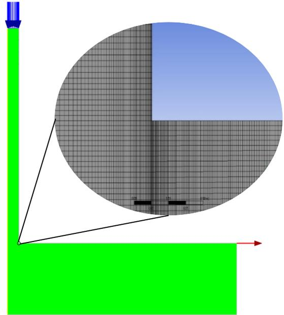
Fig. 2: Discretized mesh for the model 1 greenhouse (0° slope).
