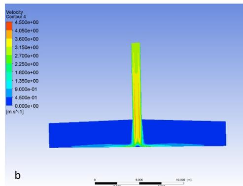
Fig. 6: The temperature (a) and velocity (b) contours of the model 2 greenhouse (0.33/90° slope).
