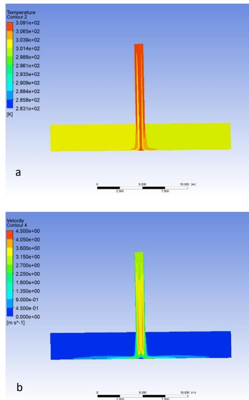
Fig. 5: The temperature (a) and velocity (b) contours of the model 1 greenhouse (0° slope).
