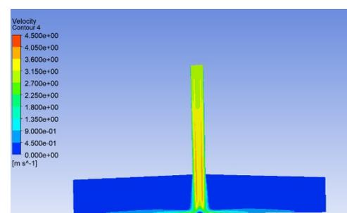
**Fig. 7:** The temperature (a) and velocity (b) contours of the model 3 greenhouse (0.5/9° slope).
