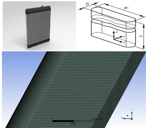
Fig. 1. Flat tube car radiator (top left), geometry of a single flat tube (top right), and the discretized mesh of the single flat tube (bottom)
