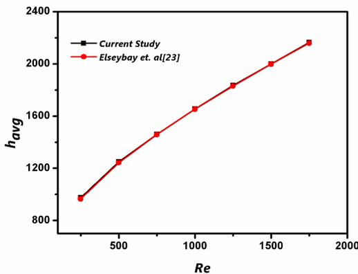
Fig. 4. Comparison of current results with those of Elsebay et al. [23] for pure water
