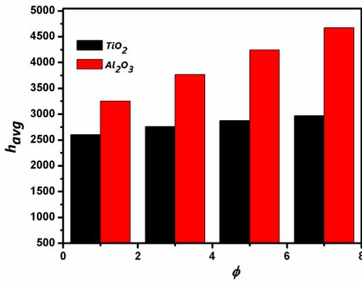
Fig. 6. Response of heat transfer coefficient for Al<sub>2</sub>O<sub>3</sub> and TiO<sub>2</sub> to the nanoparticles concentration on using two-phase approach
