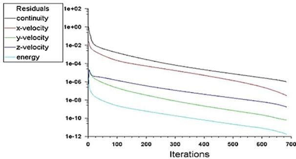
Fig. 3. Relative residual errors for the governing equations
