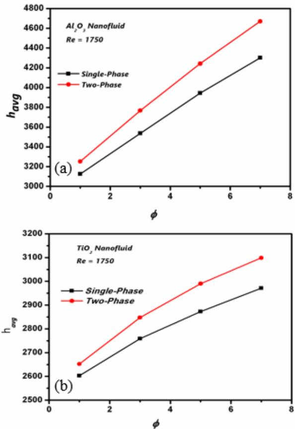
Fig. 5. The average heat transfer rate vs the nanoparticles concentration by volume for (a)  $Al_2O_3$  and (b)  $TiO_2$
