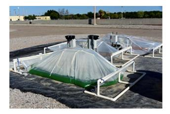
Figure 4. Field installation of the 700-L enclosed photobioreactors at the local wastewater treatment plant.
