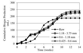
Figure 11: Biogas production from the 10% Khalas date seed/sludge mixtures
