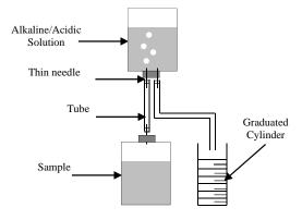
Figure 4: Volumetric total biogas and methane measurement by liquid displacement
