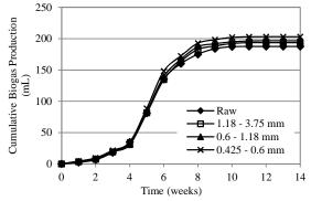
Figure 5: Biogas production from the 2.5% Khalas date seed/sludge mixtures
