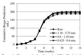
Figure 6: Biogas production from the 2.5% Khudari date seed/sludge mixtures
