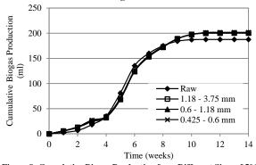
Figure 8: Cumulative Biogas Production from Different Sizes of 5% Khudari Date Seed/Sludge
