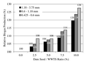
Figure 13: Relative biogas production after fourteen weeks from different khalas date seed sizes
