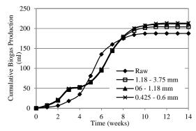
Figure 9: Cumulative Biogas Production from Different Sizes of 7.5% Khalas Date Seed/Sludge Mixtures
