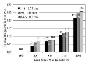
Figure 14: Relative biogas production after fourteen weeks from different khudari date seed sizes
