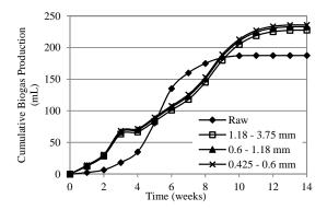
Figure 12: Biogas production from the 10% Khudari date seed/sludge mixtures
