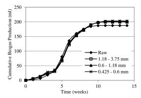
Figure 7: Cumulative Biogas Production from Different Sizes of 5% Khalas Date Seed/Sludge Mixtures
