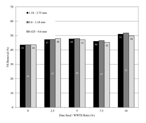
Figure 15: Volatile solids (VS) removal for Khalas date seed/sludge samples
