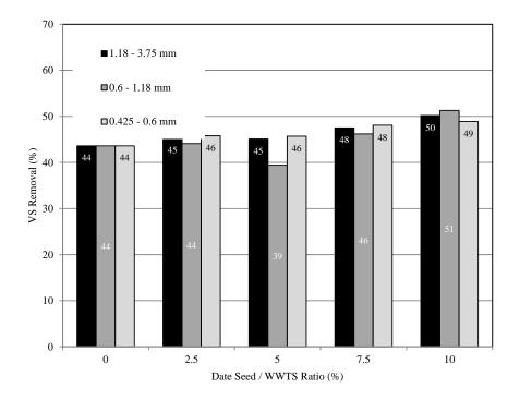
Figure 16: Volatile solids (VS) removal for Khudari date seed/sludge samples
