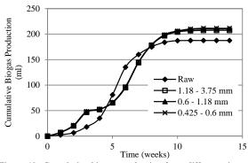
Figure 10: Cumulative biogas production from different sizes of 7.5% khudari date seed/sludge mixtures
