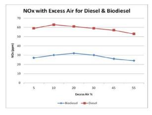
Figure 3: NO<sub>X</sub> Gas with Excess Air for Diesel & Biodiesel
