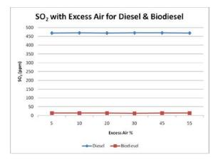
Figure 4: SO<sub>2</sub> Gas with Excess Air for Diesel & Biodiesel
