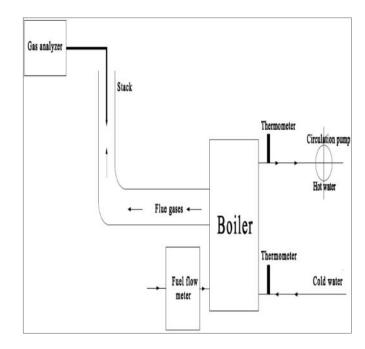
Fig. 1 Experimental Setup
