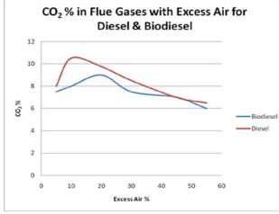
Figure 12: CO<sub>2</sub> Gas with Excess Air for Diesel & Biodiesel
