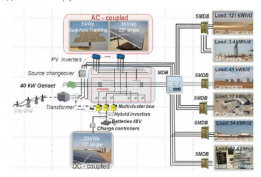
Figure 2. Line Diagram of Mingrid System
