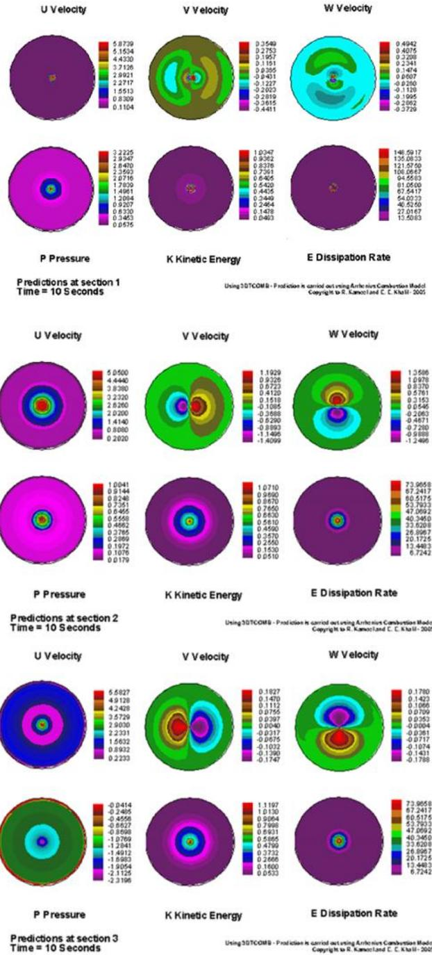
Figure 3: Predicted Flow Characteristics across the Furnace after 10 Seconds from Ignition
