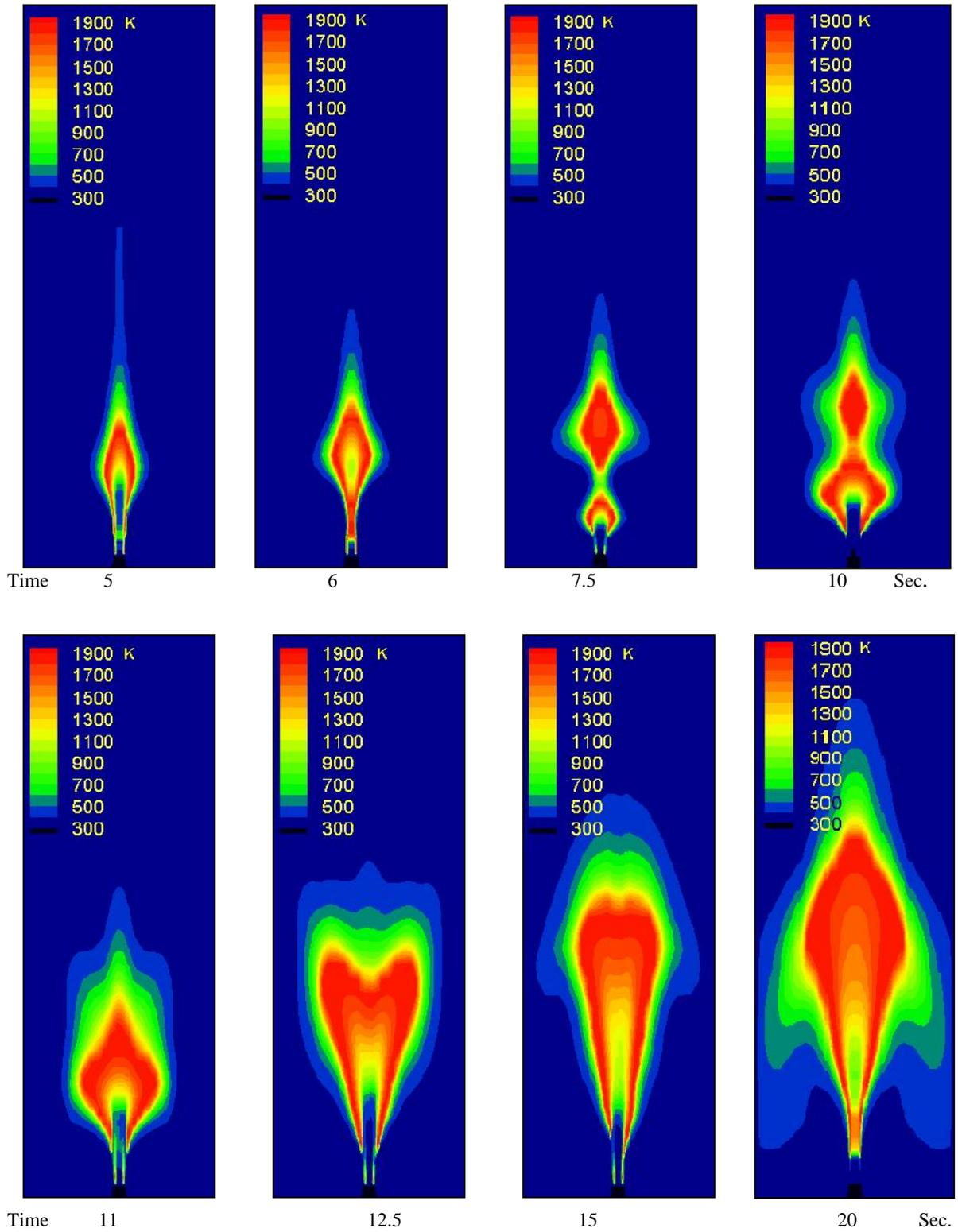
Figure 5: Predicted Temperature Contours in a Confined Flame up to 20 Seconds from Ignition
