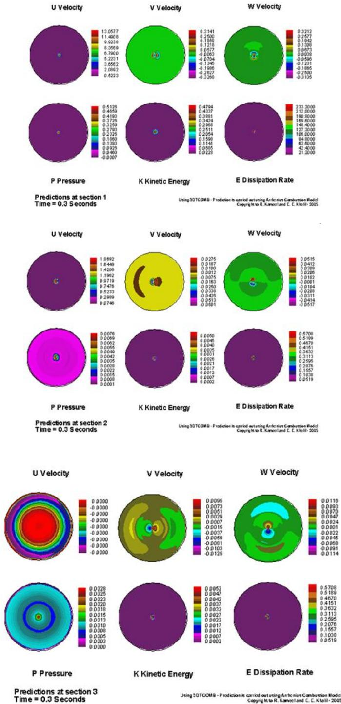
Figure 1: Predicted Flow Characteristics across the Furnace at End of Ignition
