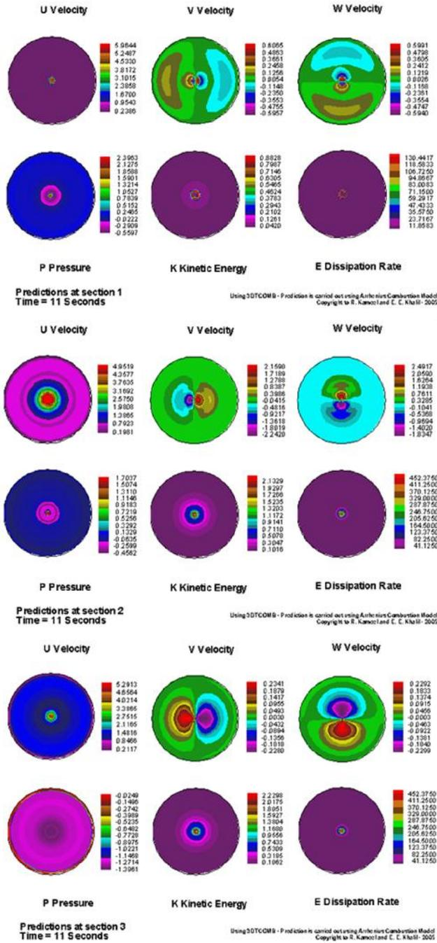
Figure 4: Predicted Flow Characteristics across the Furnace after 11 Seconds from Ignition
