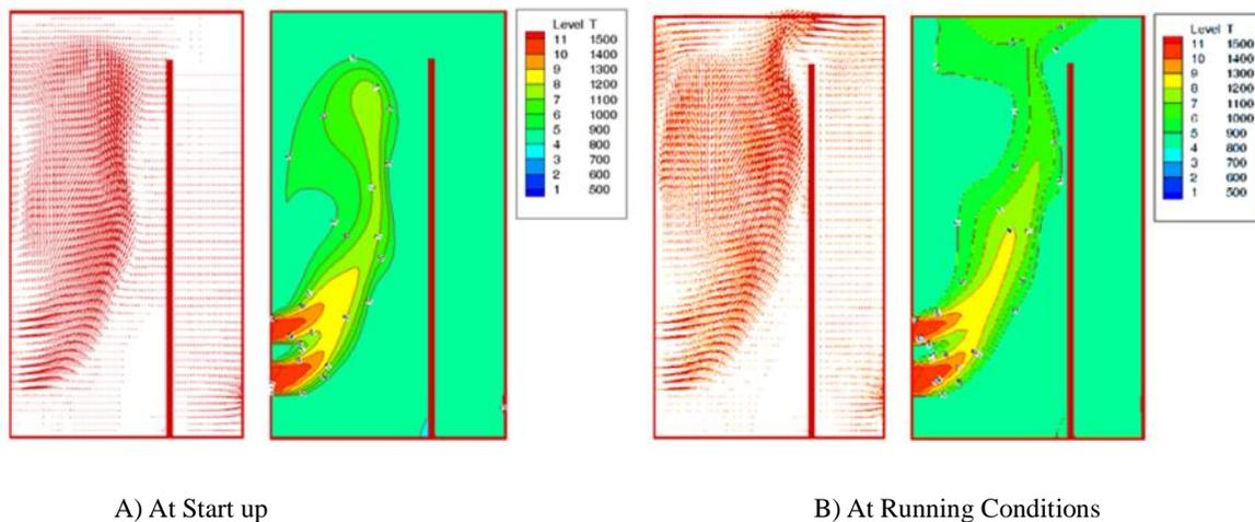
Figure 8: Predicted Time Averaged Velocity Vectors and Temperature Contours in Boiler Furnace
