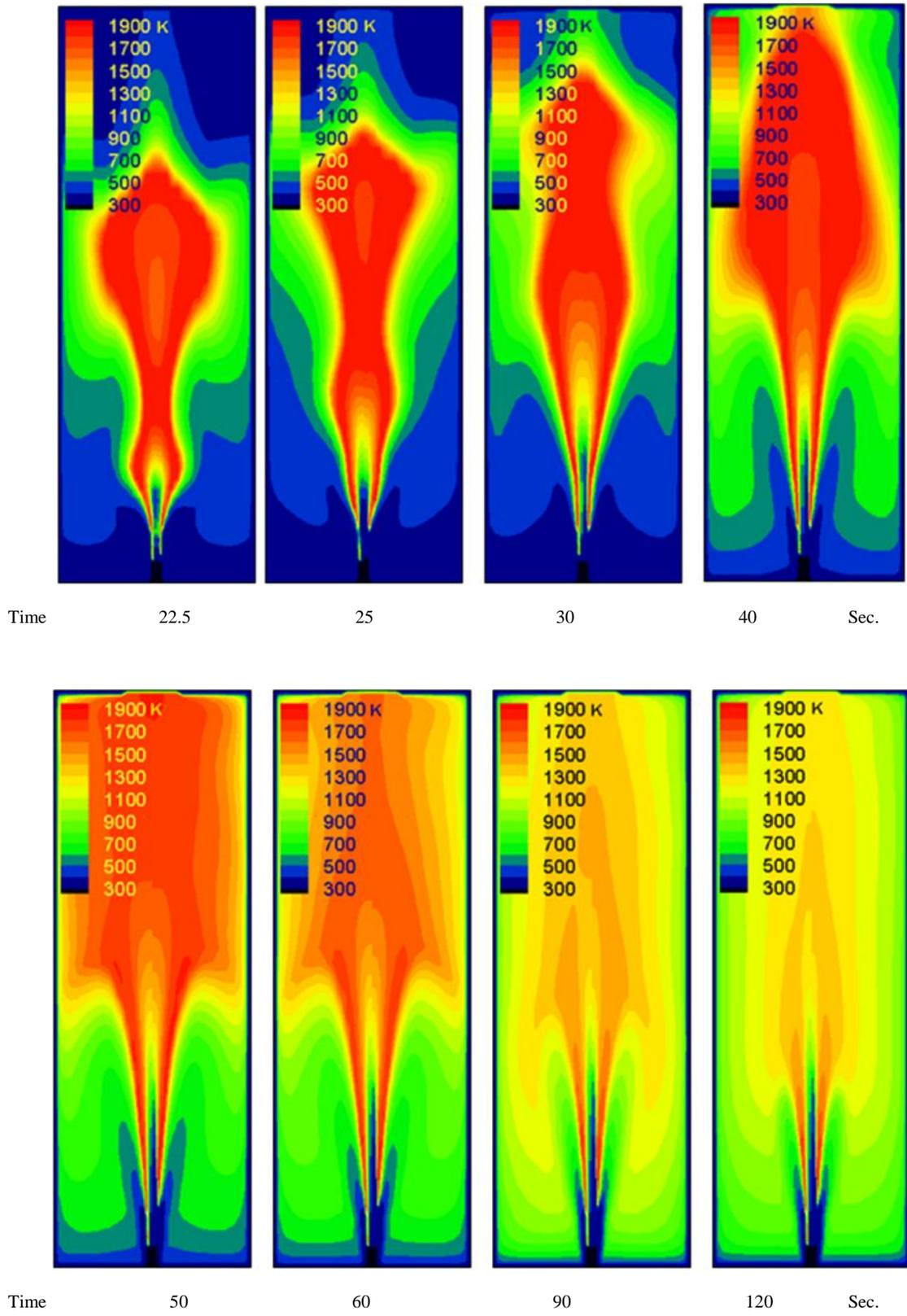
**Figure 6: Predicted Temperature Contours in a Confined Flame Up To 120 Seconds from Ignition**
