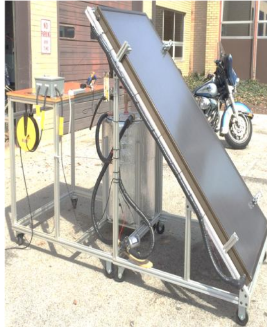
Fig. 1. Solar water heater set up
