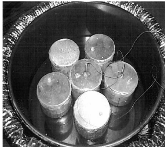
Fig. 4. Heat Exchangers inside the Water Reservoir
