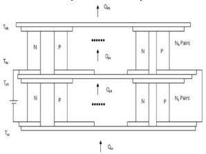
Fig. 1 Schematic diagram of the double stage TEC
