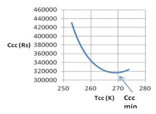
Fig. 2 Variation in cost of refrigeration produced wrt. cold side temperature
