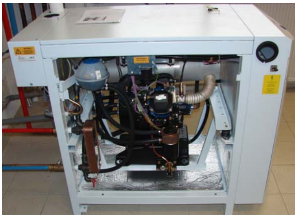
Fig. 4: The cogeneration engine.
