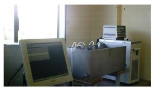
Fig. 1. ANR-100 anaerobic respirometer system.
