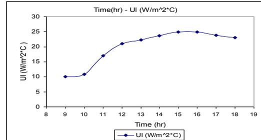
Fig. 6. Relation between overall heat loss coefficient and local standard time
