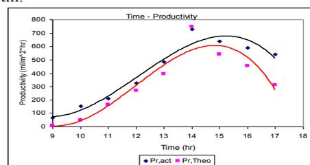
Fig. 8. Comparison between theoretical and experimental productivity of active solar still
