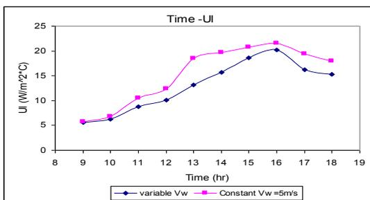
Fig. 10. Relation between local standard time and overall heat loss coefficient at different wind speeds
