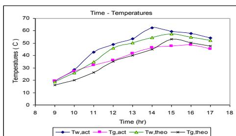
Fig. 5. Comparison between theoretical and experimental temperatures for water and glass
