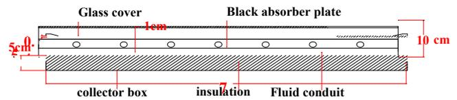
**Fig. 2. Cross section of a basic flat - plate collector**
