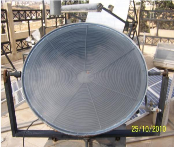
Figure 1. A two-axes tracking system, is used to maximize the incident solar radiation into the SHC.
