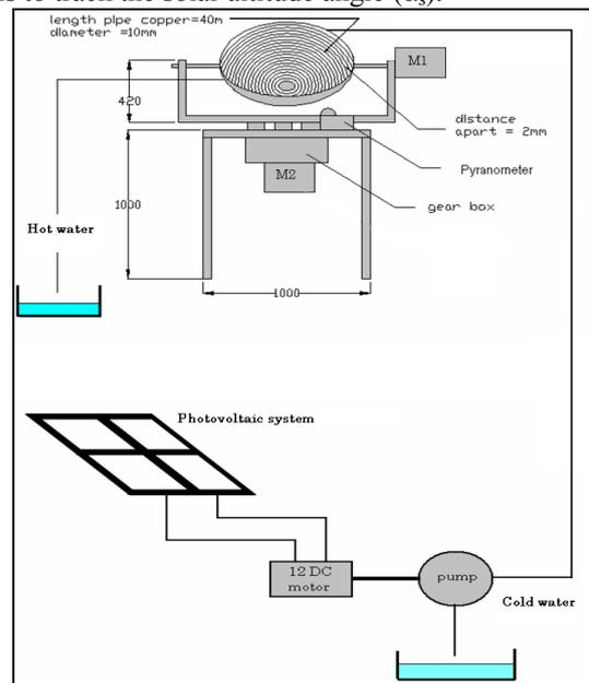
Fig. 3. The solar heating coil with a two axes tracking system
