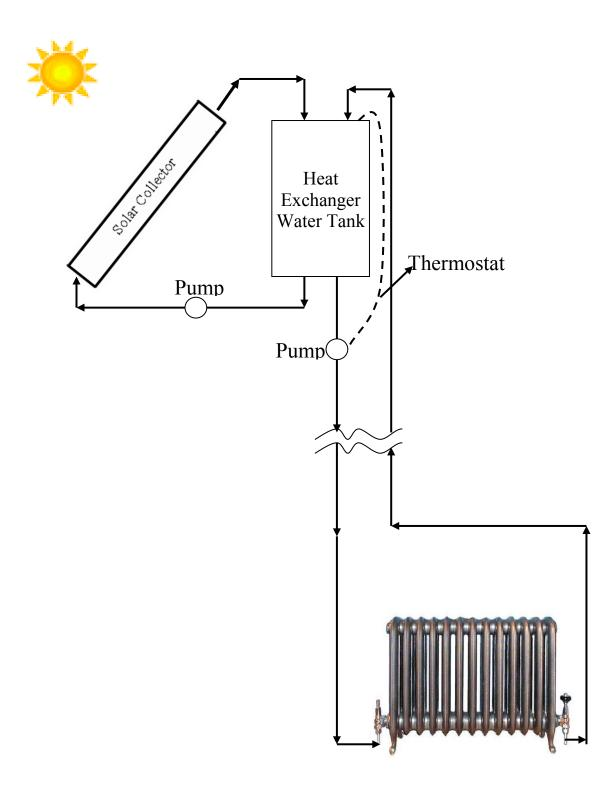
Figure 3. Schematic diagram for the proposed Heating device in the multi-apartment buildings.
