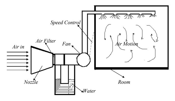
Figure 4. Schematic diagram for the proposed cooling device in the multi-apartment buildings.
