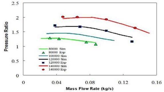
Fig. 14. Comparison between simulated and measured mass flow rates at varying turbocharger speeds using through-flow model [11]
