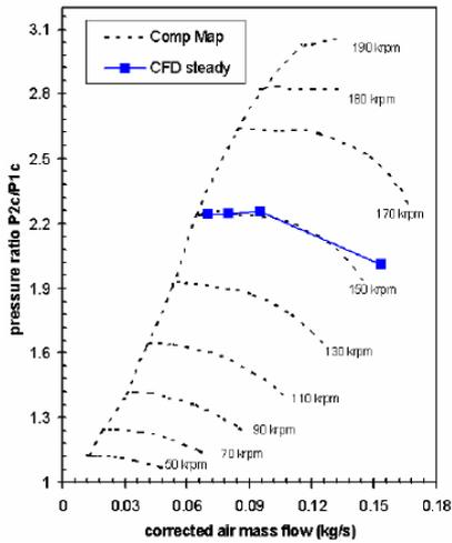
Fig. 9. Compressor flow map created by experimental data [7]
