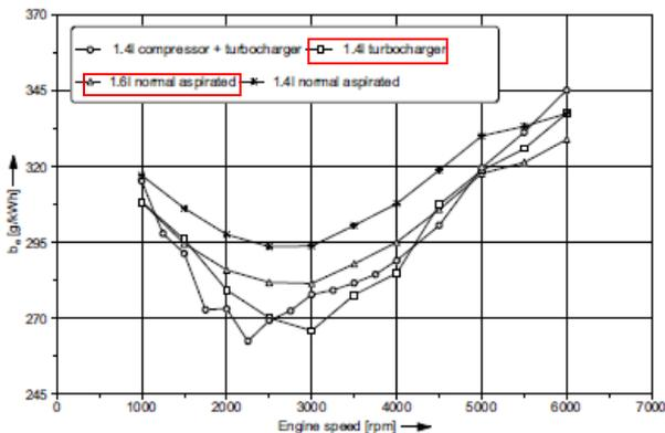
Fig. 17. Comparison of fuel consumption between four different engine configurations [13]
