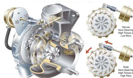
Fig. 19. Variable geometry turbocharger ([www.volvo.com](http://www.volvo.com))
