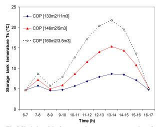
Fig. 5. Variation of the Storage tank temperature versus time of day for various values of the couple  $A_{\rm C}/V_{\rm S}$
