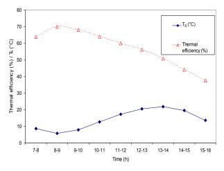
Fig. 6. Variation of the Storage tank temperature and thermal efficiency of solar collectors versus time of day
