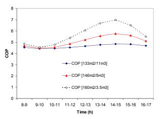
Fig. 3. Variation of the COP versus time of day for various values of the couple  ${\bf A}_C/V_S$
