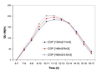
Fig. 4. Variation of the of collected heat versus time of day for various values of the couple  ${\bf A}_C/V_S$
