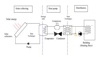
Fig.1. Schematic diagram of solar assisted heat pump system
