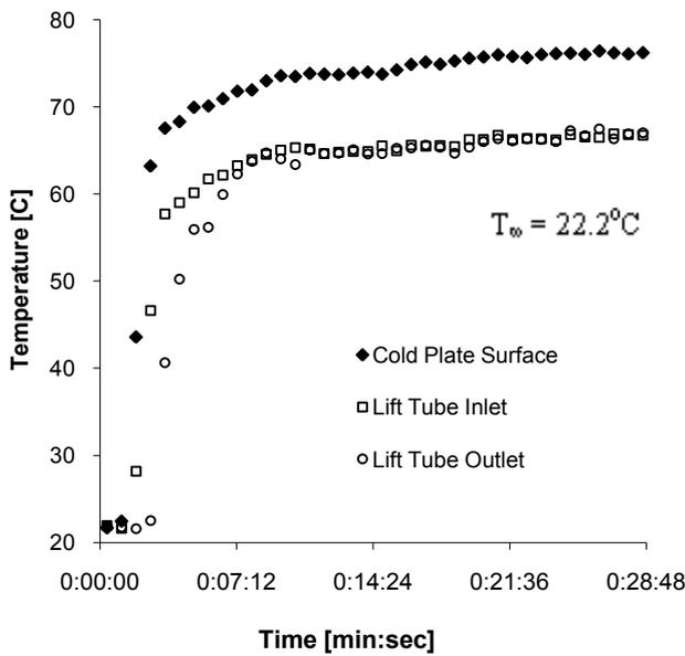
Fig.8. Performance of bubble pump for heating load of 400 W
