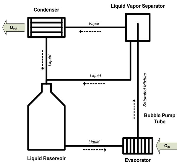
Fig.1. Schematic of the bubble pump cooling system
