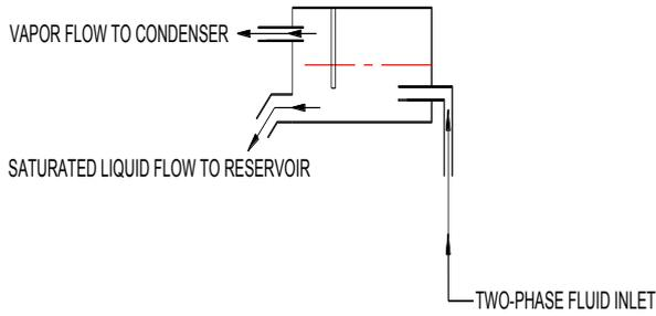
Fig.2. Schematic diagram of the inline separator
