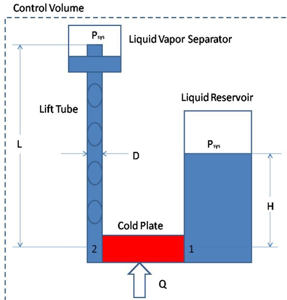
Fig.3. Bubble pump schematic
