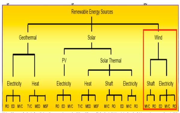
PV = Photovoltaic Solar, RO = Reverse Osmosis, ED = Electrodialysis, MVC = Mechanical Vapor Compression, MED = Muti-Effect Distillation, Multi-Stage Flash Distillation, TVC = Thermal Vapor Compression
