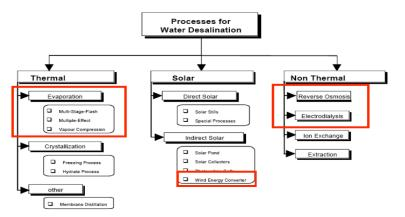
Fig. 2. Categories of Desalination Processes
