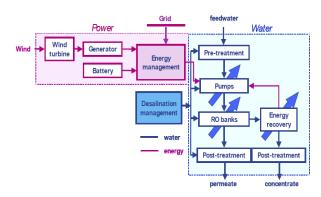
Fig. 9. Components of system model for wind-powered RO. [41]
