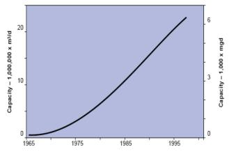
Fig. 5. Total Installed Capacity of Desalting Facilities [33]
