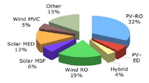
Fig.8. Distribution of Renewable-Powered Desalination Technologies [36]
