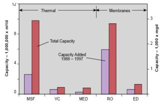
Fig. 6. Distribution of Desalination Capacity by Type of Technology [33]
