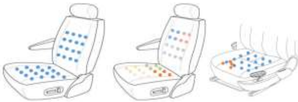
Fig. 3. Distribution of Force Sensors Using Normal Distribution Without Grouping or Dividing into Areas (Left), Distribution of Force Sensors by Dividing Sensors into Areas According to Different Approaches (Middle), and Distribution of Sensors with the Addition of Four Additional Sensors for Brake and Accelerate Posture (Right) [16]
